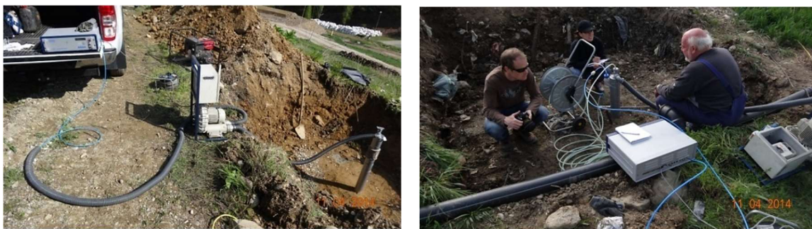
Fig. 17.8 a+b Sucking from the top and measuring in different depths
