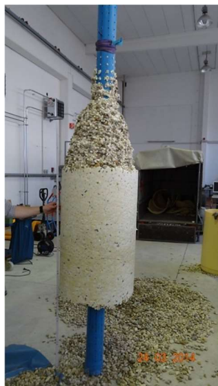
Fig. 17.6 a+b Foam body of a restored gas well in the laboratory test
