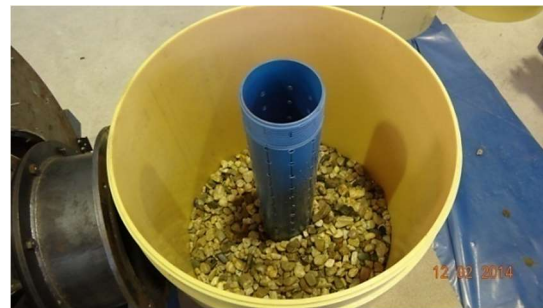
Fig. 17.5 a+b Model of a gas well in the laboratory
