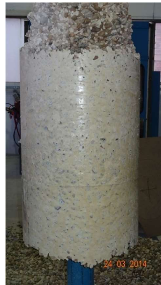
Fig. 17.6 a+b Foam body of a restored gas well in the laboratory test
