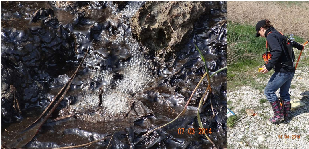
Fig. 17.1 a+b Bubbles of methane at the surface of a landfill and measuring of gas on the surface of another landfill (LUBW 2008)
