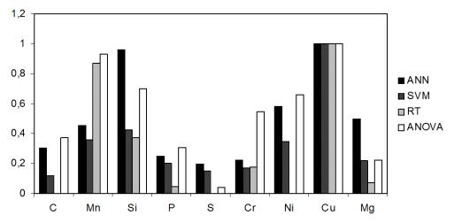
Fig. 10.5 Relative significance factors for the industrial data set (tensile strength of ductile cast iron vs its chemical composition defined by 9 elements) obtained from regression models using various learning systems and ANOVA [18]
