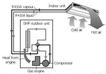
Fig. 9.1 Operation principle of gas heat pump GHP AISIN in heating mode
