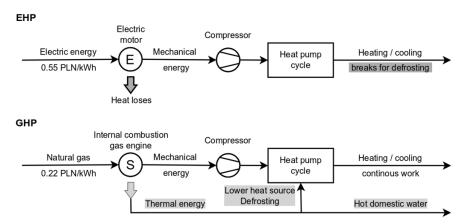
Fig. 9.3 Energy utilization in electric (EHP) and gas (GHP) heat pump systems
