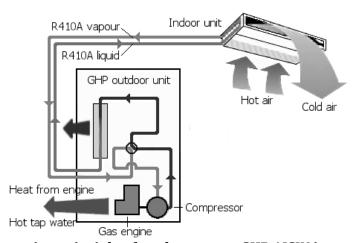
Fig. 9.2 Operation principle of gas heat pump GHP AISIN in cooling mode
