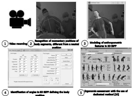
Fig. 1.8 The track of video frames processing for the ergonomic assessment
