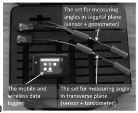
Fig. 1.1 The recording means a) digital camera Sony, b) the set for the wireless measuring body position
