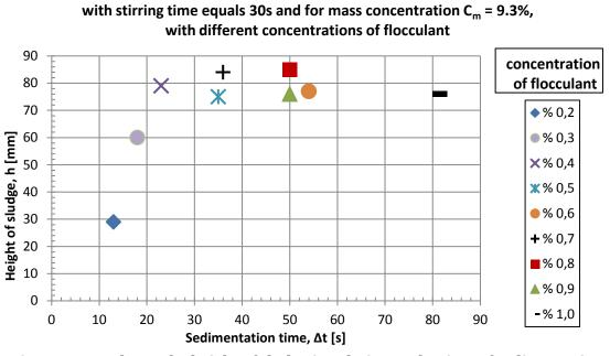
The height of sludge in relation to sedimentation time of hydromixture
