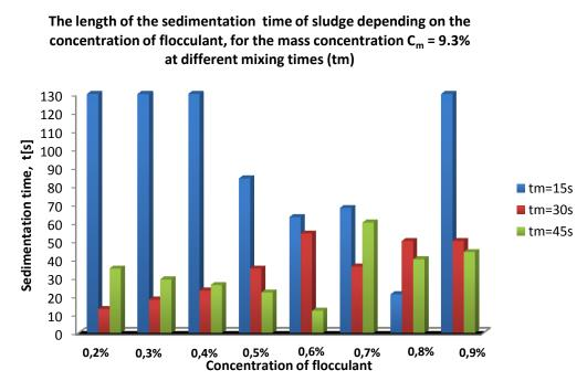
**Fig. 7.2 Time dependence of sedimentation sludge from concentration of added flocculant** Source: own study
