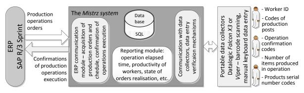
Fig. 6.2 Data acquisition in Mistrz system
