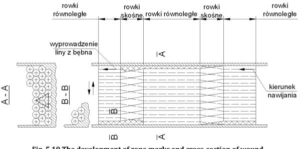
Fig. 5.10 The development of rope marks and cross-section of wound layers in LeBus synchronous method [4]
