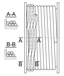
Fig. 5.2 Two-layer winding of rope on cylindrical drum with lining with helical grooves [13]
