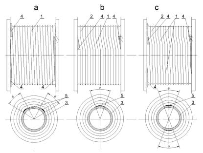
Fig. 5.1 Types of grooving the lining of cylindrical drums [14]:
