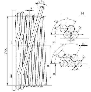
Fig. 5.5 Diagram of the rope transition from coil to coil during multi-layer winding on cylindrical drum with helical grooves [7], I-I the first transition (the first pitch), II-II – second rope transition (the second pitch)
