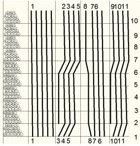
Fig. 5.3 Development of surface of the winding of drum lining with spiral grooves [4]
