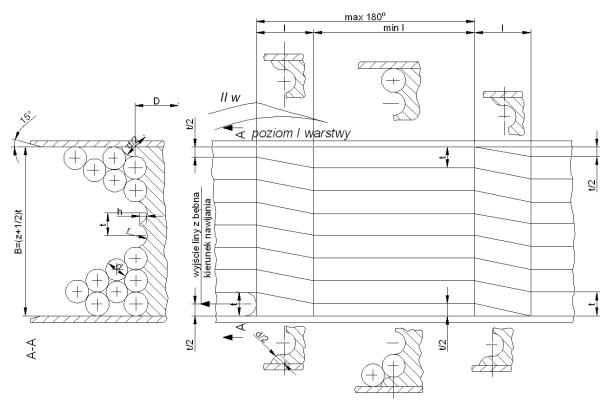
Fig. 5.9 Winding, using the synchronous LeBus method [4]
