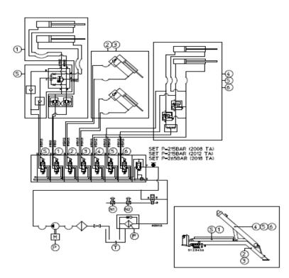
Fig. 14.7 Hydraulic scheme of a skiploader [9]: 1 – system of arm rotation cylinders with a section of the control valve controlling arms' rotation, 2, 3 – stabilizer cylinders and responding of them sections of the control valve, 4, 5, 6 – telescopic arm cylinders and responding of them sections of control valve,
