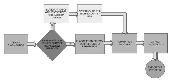
Fig. 14.5 Algorithm of activities of a company authorised for performing reparations and modernisations of handling equipment [8]
