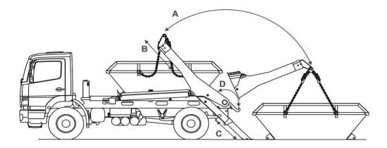
Fig. 14.2 Working movements of a skiploader [3]: A – Tipping boom for loading and unloading the container, B – Telescopic boom extending and retracting, C – Stabilizers extending and retracting, D – Tipping hook opening and closing (pneumatic movement)
