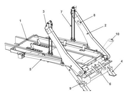
Fig. 14.1 Skiploader [3]: 1 – platform, 2 – tipping arm, 3 – telescopic boom, 4 – stabilizer, 5 – tipping cylinder 6 – tipping hook, 7 – chain, 8 – telescopic arm cylinder, 9 – stabilizer cylinder, 10 – pneumatic cylinder of tipping hook
